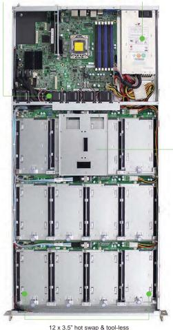
2-bay 2.5" drive bracket is in the middle when using redundant PSU -
